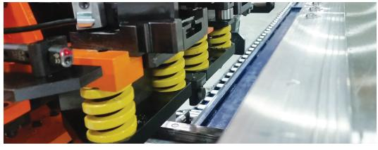
A major truck trailer manufacturer reduced a portion of their assembly costs by 98 percent using a Tog-L-Loc® clinching machine, custom designed and built by BTM Company. Previously, the manufacturer used self-piercing rivets to attach the roof to the two long side walls and front section of the trailer. BTM's Tog-L-Loc® clinching machine dramatically reduced the number of rivets required in this portion of the manufacturing process, netting huge cost-savings for the manufacturer.
