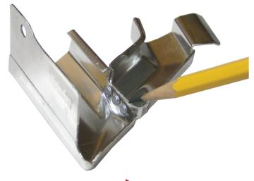
A custom Multi-Clinch® three joint die like the example shown here clinched the automotive window trim section shown above.
